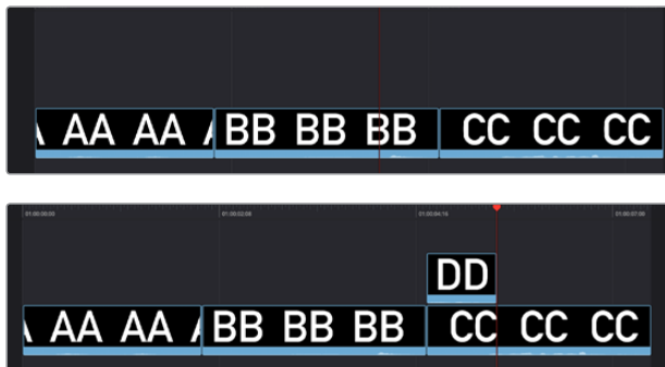
(Top) Before a Close Up edit, (Bottom) After editing clip DD into the Timeline with a Close Up edit Place on Top
